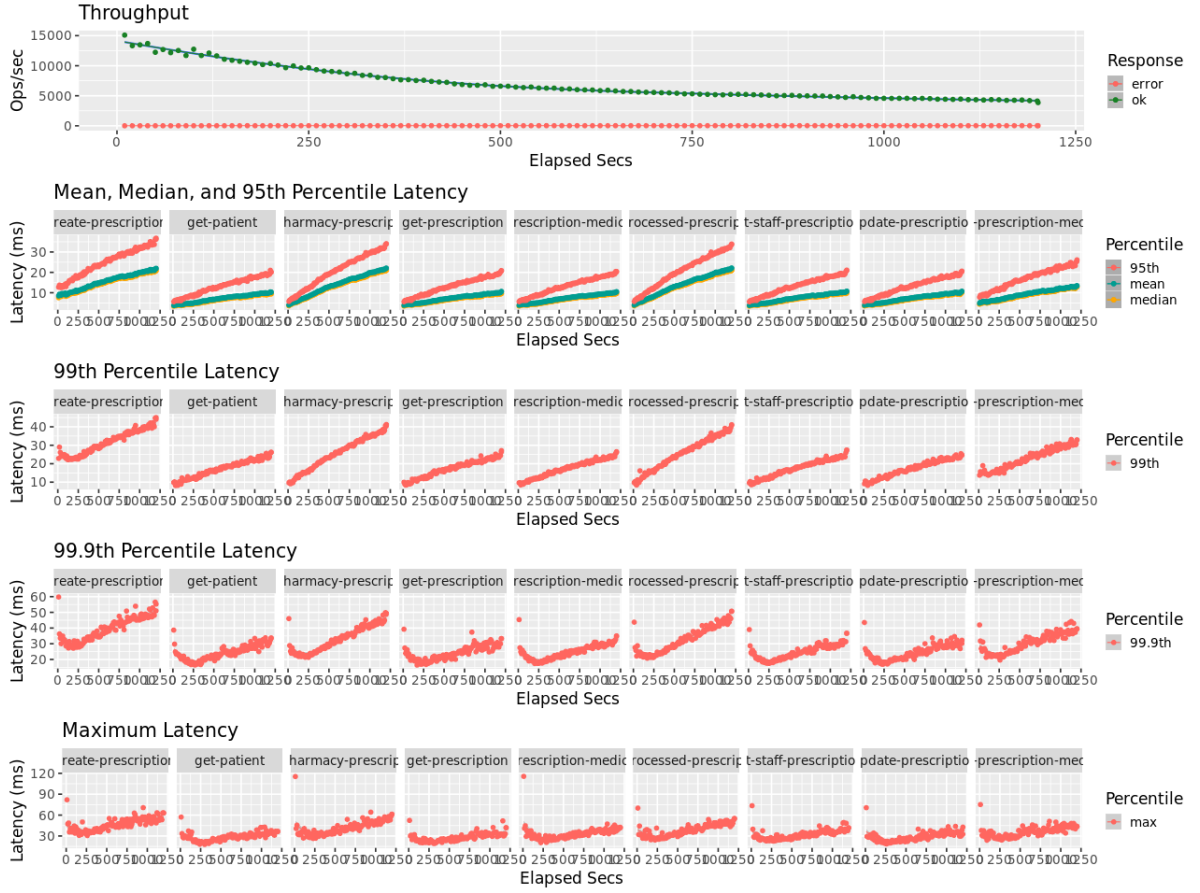
Figure 5.6: Throughput over latency plot using 64 clients
